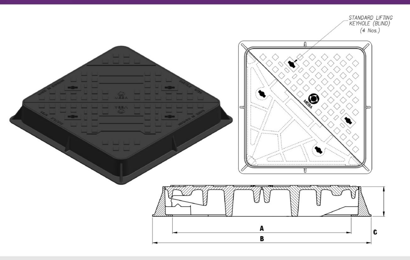
Features: Heavy duty ductile iron manhole cover and frame.
